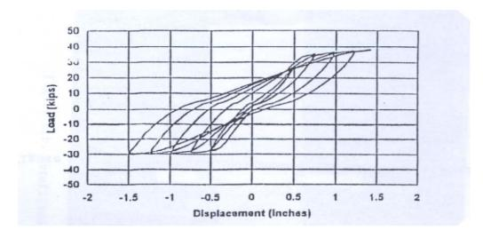
Figure-1 Load-Deflection plot for the control specimen SP-1
