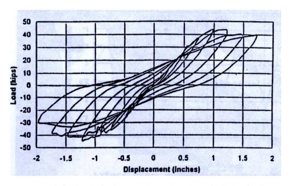
Figure 2 Load-Deflection plot for the repaired control specimen with E-glass SP-1R
